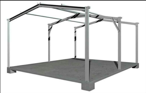
2B COMPLETE PORTAL FRAME ASSEMBLY REFER 2C FOR TEMPORARY BRACING LOCATION
