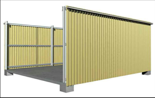
1B SECOND SIDEWALL FRAME REFER 1C FOR TEMPORARY BRACING LOCATION
